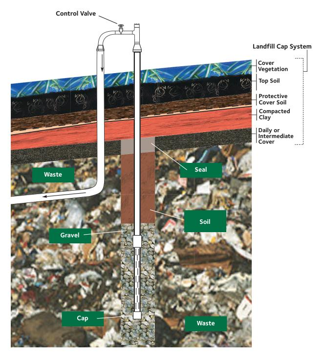
Gas extraction wells are used to collect gas that is generated as the waste decomposes. The gas is used to produce energy or is sent to a flare.
